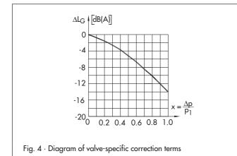
Terms for control valve sizing according to DIN EN 60534, Parts 2.1 and 2.2: F1 = 0.95
